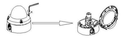
2. Set the mounting base onto the wall or ceiling and center it over the mounting hole, using the supplied four retaining screws to secure the main body.
